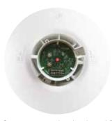
Cover removed showing LED self diagnostics and optional functionality buttons of flow rates fine tuning. This function can be very useful during commissioning.
